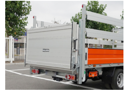
OVT110.1 - Aluminium platform of the DH-VO& K1 / VB& E1 in anodised finish
