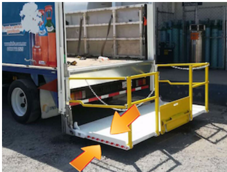
Lateral fall-off protection
