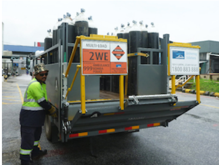
Automatically folding guard rails (here shown on a hydraulic closure lift [option OVH004])
