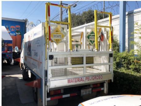
Air-permeable platform with steel grids. Reduces wind-resistance, improves fuel consumption and anti-slip protection.
