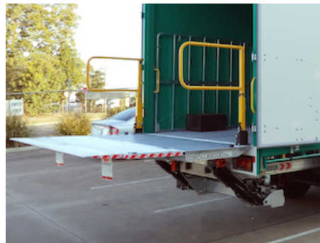
OAP203.LR - 2 hinged safety rails on foldable platform
