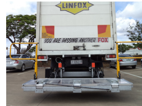
OAP204.LR - 2 safety rails with rotating foot
