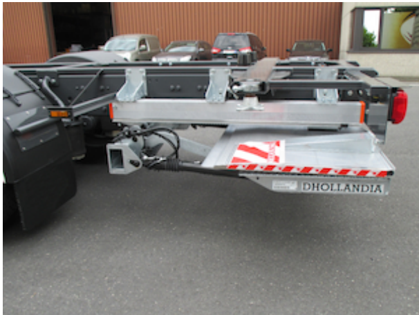
Truck: aluminium sliding tubes with bolt-on mounting brackets for quick fitting to truck chassis
