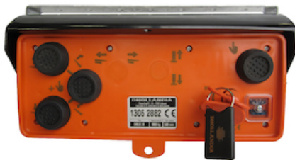
Arctic exterior control box with IP67 rated sealed contacts, and a main battery isolator switch with removable key [OAE041.BP]
