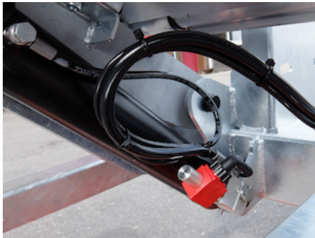
Manual emergency operation on all electrovalves
