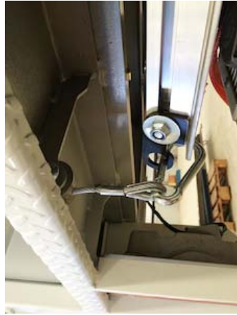
OAP620.C - Platform lock DH-RP with steel rope
