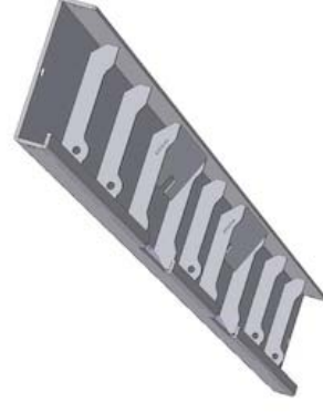
OAM004 - Rear floor traverse RP06/RP10 (tear plate)
