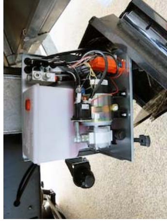
Robust pump unit 12V or 24V DC mounted at the side of the lift frame
