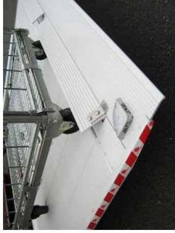
OAP100.M - Manual rollstops in platform point
