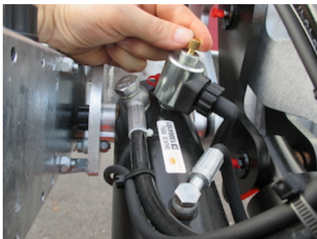
Manual emergency operation on all electrovalves
