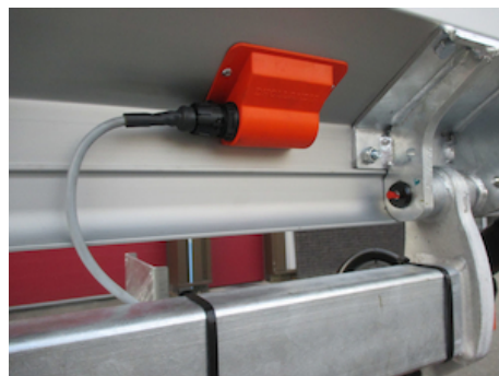
OAE502 - Reed sensor on platform
