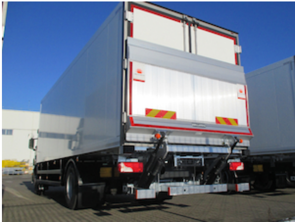
Light-weight aluminium platform with anti-slip surface
