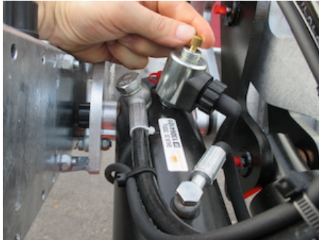
Manual emergency operation on all electrovalves
