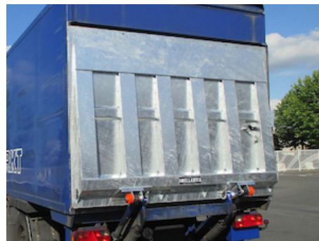
OAT124 - GALVA finish for steel DHL* platform
