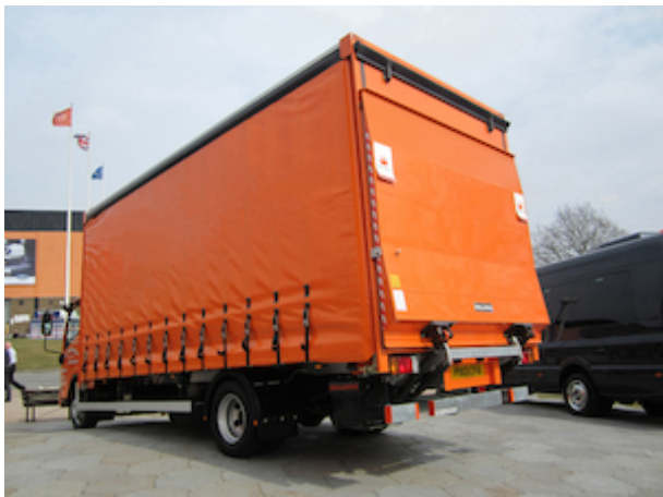
Tail lift for 1000-1500 kg lift capacity with minimal proper weight, offers maximum pay-load on trucks of 7.5-12T GVW
