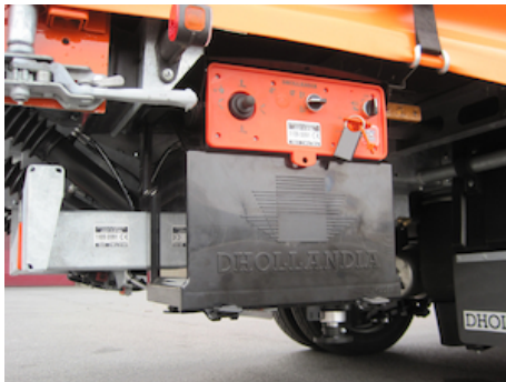
Control unit integrated in cover of pump unit, with main battery isolator switch and removable key [OAE039.BP]
