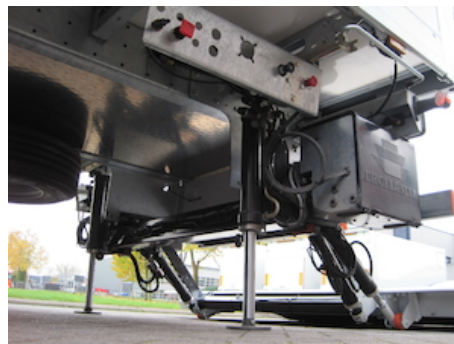
OAH013.60.LE - Hydr.stabilising leg straight 4T LE...mm
