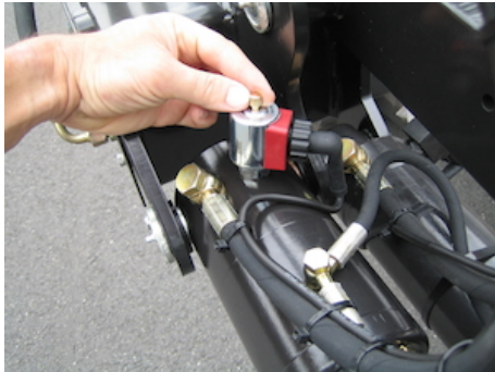
Manual emergency operation on all electrovalves
