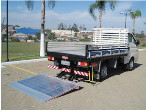
Light-weight aluminium platform with anti-slip surface
